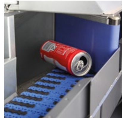
The switch actively deflects the container
