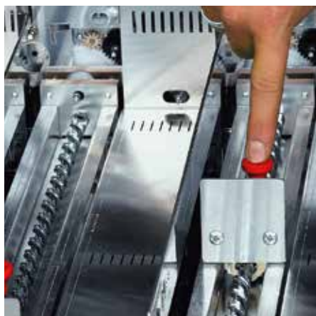
Multiflex pushers to dispense larger products, available in different sizes
